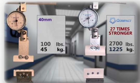
Pull-Apart Strength Test with 152mm (6in.) Sample. Qcompact Pull Apart at 8050 kg/m 40mm Pull Apart at 296 kg/m
